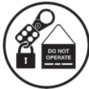
Figure 11. Ensure there is a Safety Protection Guarantee or lockout in place and check that it is appropriate for your work
