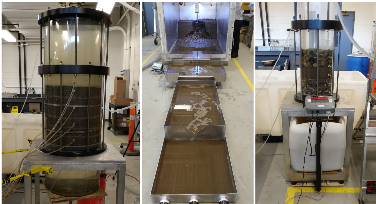
Figure 11 Newly developed and commissioned apparatus for Internal Stability Test (left), Crack Holding Test (center), and Continuing Erosion Filter Test (right) at Powertech Labs, developed under the Large Embankment Dams Special Investigations.
